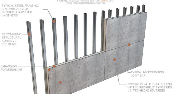
FASTEN on EACH SIDE PASLODE NAIL 2 - 1/2" L x 0.131" DIA. SMOOTH SHANK at 4" o.c. and 3/8" BEAD ADHESIVE or 15 ga. 11/2 STAPLES @ 3" o.c.
